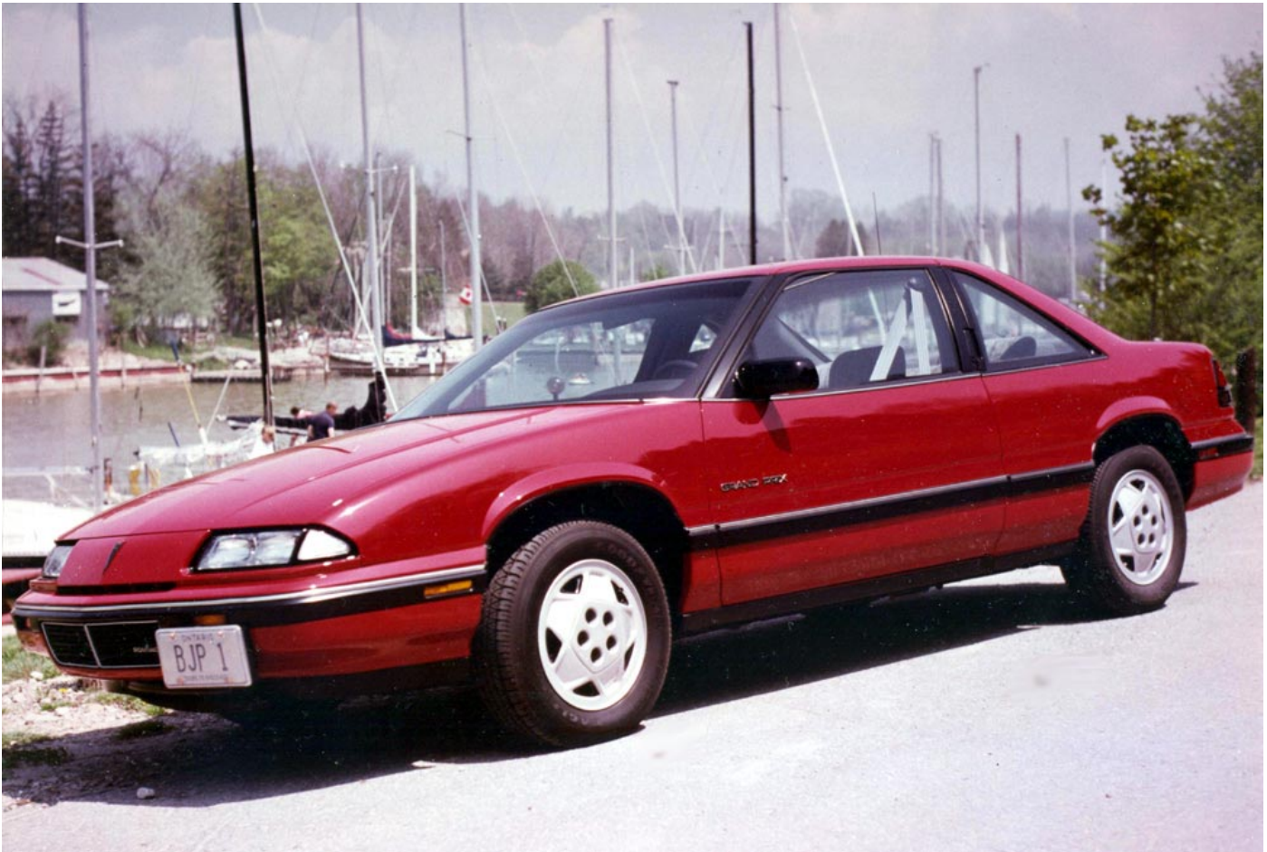
1988 Model Pontiac Grand Prix Coupé. The Base Model Grand Prix was Powered by a 2.8 litre V-6 Multi-port Fuel-injected Engine Coupled to a Manual Five-speed Transaxle and Front Wheel Drive. I had Reverted to a Single Colour Paint – Metallic Red, and the Optional Extra Features Included Air Conditioning, Cruise Control and an FM Radio with Cassette Tape Player. The Instrumentation Displays were in both Analog and Digital Formats. Photograph Taken Outside the Bayfield Marina, Ontario, in May, 1988.
