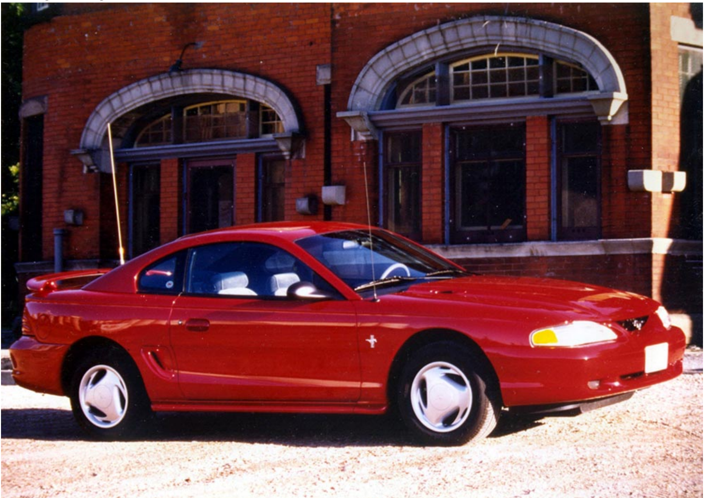
1994 Model Ford Mustang Coupé. The non-GT Mustang was Powered by a 3.8 litre V-6 Sequential Multi-port Electronic Fuel-injected Engine Coupled to a Manual Five-speed Overdrive Transaxle and Rear Wheel Drive. The Colour was Described as Laser Red Tinted Clearcoat Metallic, and the Optional Extra Features Included Air Conditioning and an FM Radio with Cassette Tape Player. The Instrumentation Panel was Fully Equipped. Photograph Taken Outside the 1907 CPR Station, Goderich, Ontario, in July, 1994.
