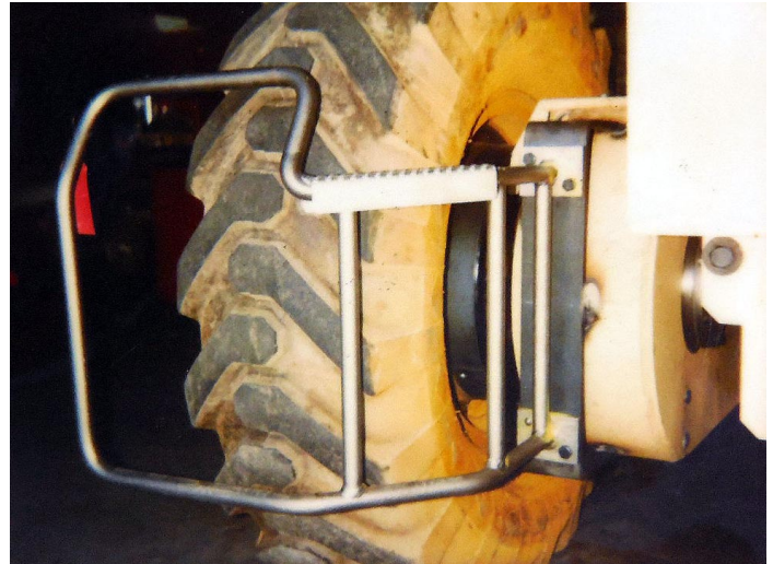
Prototype Tire Guard Installation for the Japanese Motor Graders per Barry's Design, July, 1991.
