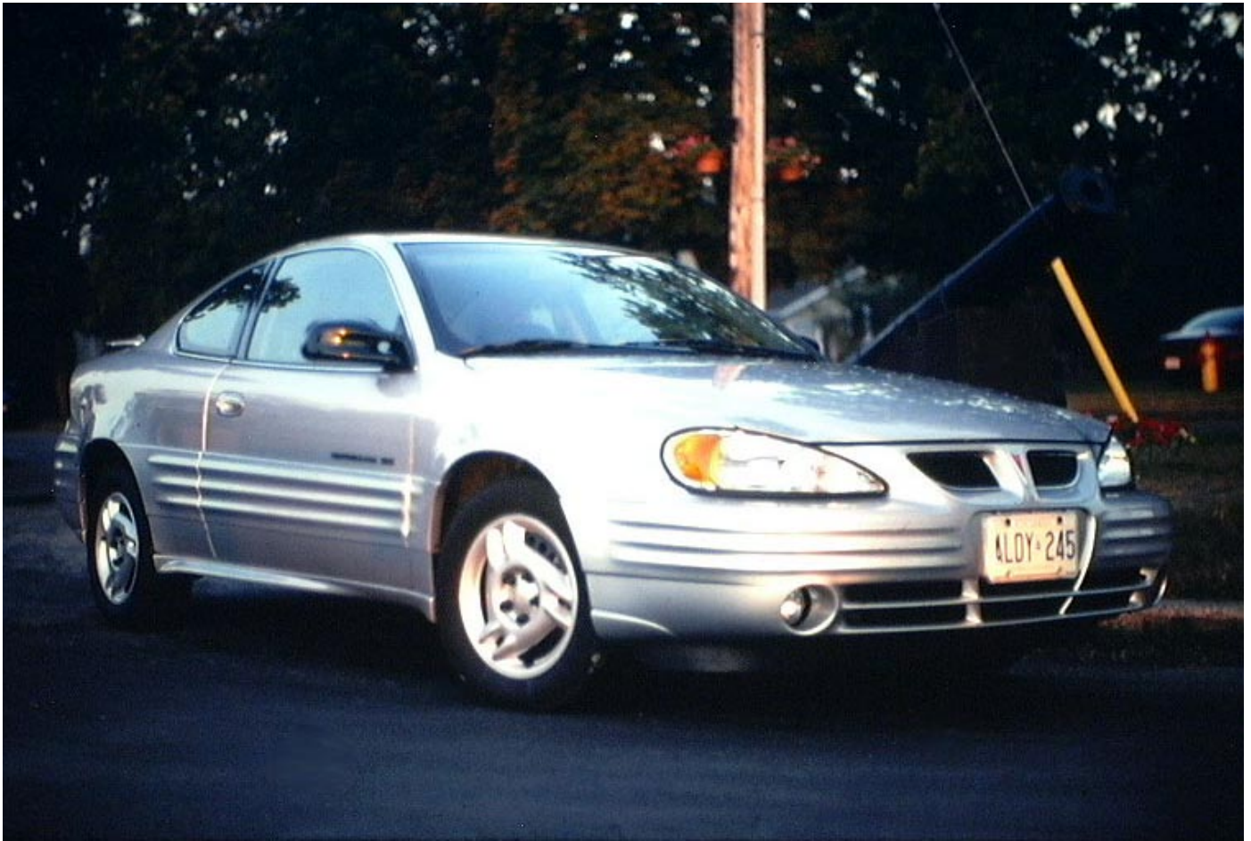
2001 Model Pontiac Grand AM SE Coupé. The Base Model Grand AM was Powered by a 2.2 litre Inline 4-Cylinder Sequential Fuel-injected Engine Coupled to a Manual Five-speed Overdrive Transaxle and Front Wheel Drive. The Colour was Described as Galaxy Silver Metallic, and the Optional Extra Features Included Air Conditioning, Cruise Control and CD Player. The Instrumentation Panel was Fully Equipped. Photograph Taken at the Lighthouse Turnaround of Cobourg Street, Goderich, Ontario, in September, 2002.
