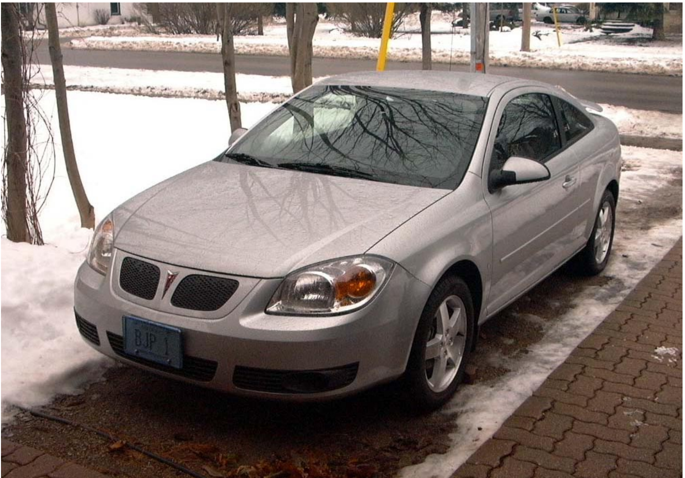
2006 Model Pontiac Pursuit SE Coupé. This Model Pursuit was Powered by a 2.2 litre Inline 4-Cylinder Sequential Fuel-injected Engine Coupled to a Manual Five-speed Overdrive Transaxle and Front Wheel Drive. The Colour was Described as Ultra Silver Metallic, and Standard Features Included Air Conditioning and Cruise Control. The CD Player was an Optional Extra and the Instrumentation Panel Had Basic Gauges. Photograph Taken Outside our Cambria Road Apartment, Goderich, Ontario, in December, 2005.
