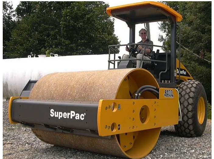
Barry Operating a SuperPac Model 8400 Road Roller at the Test Site, Asheville, North Carolina, June, 2004.
