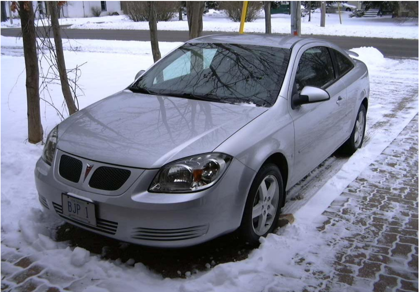
2009 Model Pontiac G5 SE Coupé. This Model Superseded the Pursuit and was Powered by a 2.2 litre Inline 4-Cylinder Sequential Fuel-injected Engine Coupled to a Manual Five-speed Overdrive Transaxle and Front Wheel Drive. The Colour was Described as Quicksilver Metallic, and Standard Features Included Air Conditioning, Cruise Control and CD Player. The Instrumentation Panel Had Basic Gauges. Photograph Taken Outside our Cambria Road Apartment, Goderich, Ontario, in December, 2008.
