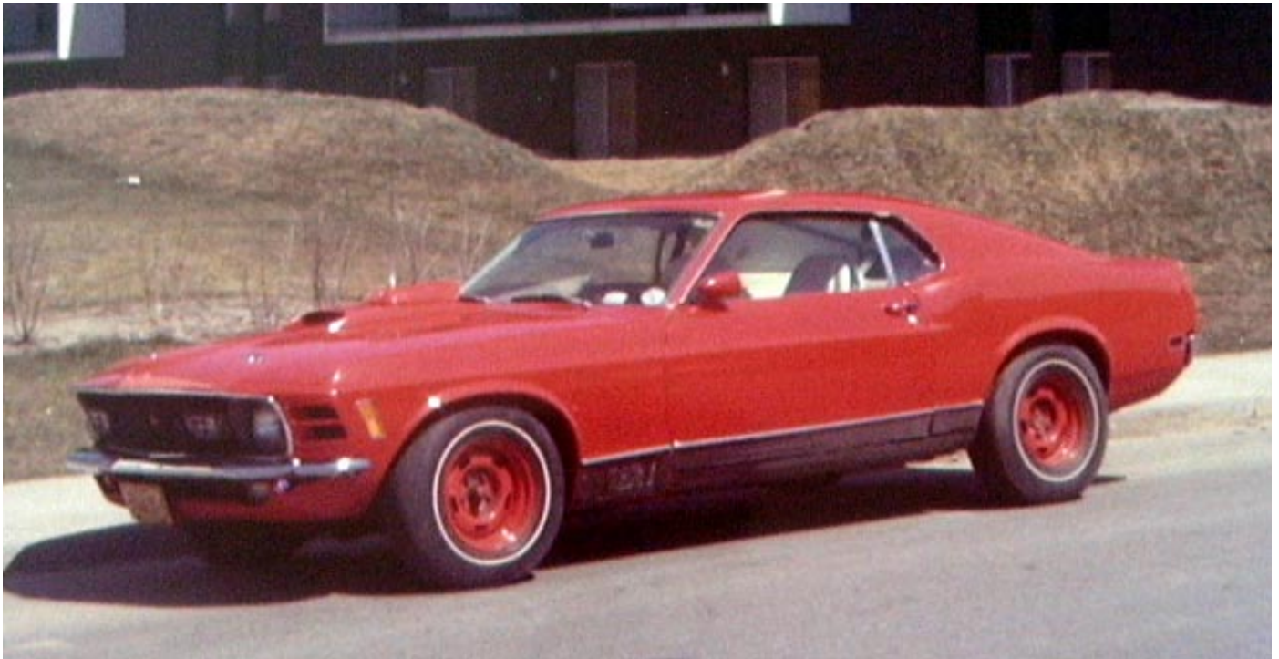
1970 Model Ford Mustang Mach 1 Sports Coupé. It was Powered by a 428 cu. in. Cobra Jet V8 Engine with a 4 Barrel Carburettor (Carburetor).
