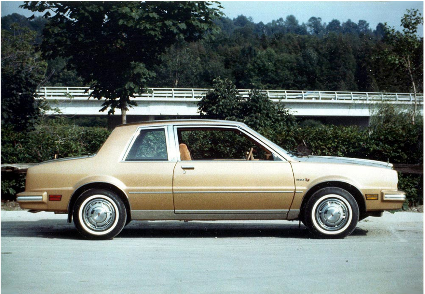
1980 Model Pontiac Phoenix LJ Coupé. It was Powered by a 2.8 litre V6 Engine Coupled to a Manual Four-speed Transaxle and Front Wheel Drive. One of the New GM 'X' Body Cars that Included the Buick Skylark, Chevrolet Citation, Oldsmobile Omega and Cadillac Cimarron. Photograph Taken Outside the River Mill Annex to the Benmiller Inn, Benmiller, near Goderich, Ontario, in the Summer of 1979.
