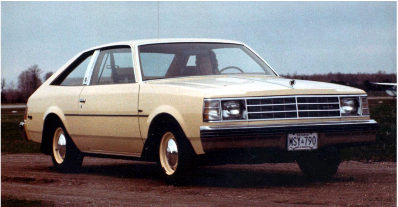
1978 Model Buick Century Coupé. It was Powered by a 3.2 Litre V6 Engine Coupled to a Three-speed Automatic Transmission. Photograph Taken Outside the Business Air Services Hangar at Sky Harbour Airport, Goderich, Ontario, in the Spring of 1978.
