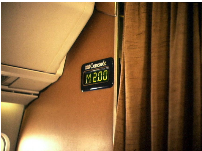
The Machmeter Indicates that Concorde is Flying at Supersonic Speed – over the Atlantic, Sept., 1981.
