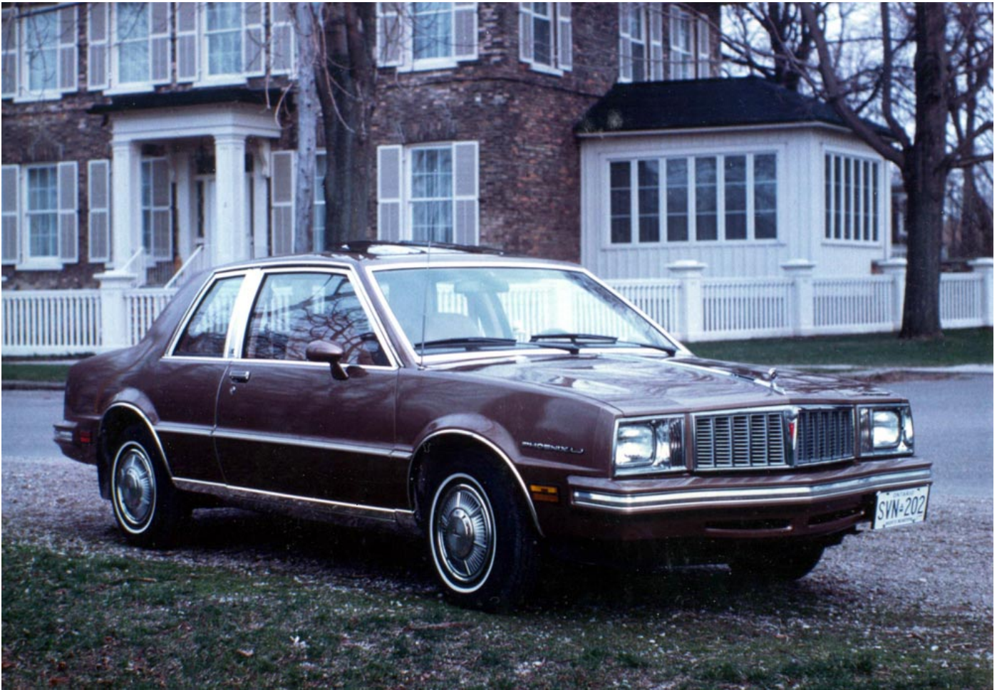
1982 Model Pontiac Phoenix LJ Coupé. This Redesigned Car was Once Again Powered by a 2.8 litre V6 Engine Coupled to a Manual Four-speed Transaxle and Front Wheel Drive. An Additional Refinement was the Removable Sunroof Panel, and the Passenger Side Mirror was an Optional Extra. Photograph Taken Outside the Home of Mr. Bruce Sully, CEO of Champion Road Machinery Ltd., Goderich, Ontario, in the Spring of 1982.
