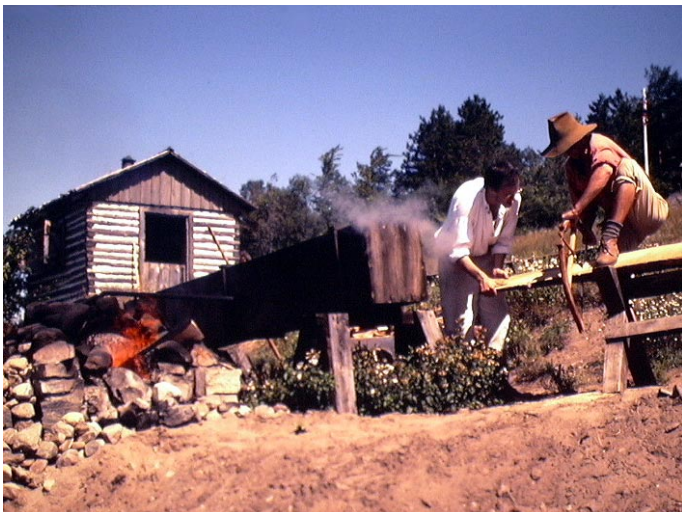
Craftsmen Using a Steam Box to Bend Wood at the Navy Yard, Penetanguishene, Ontario, August, 1984.
