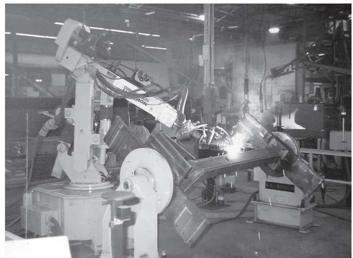
Champion's New Welding Robot Undergoing Test Trials, Goderich, Ontario, October, 1986.
